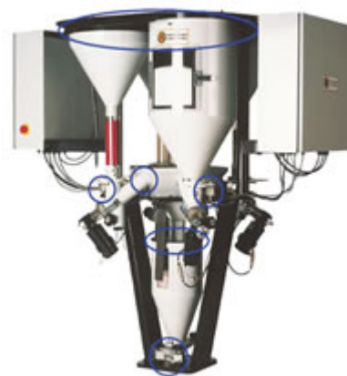
Fig. 2—An X-Series continuous blender, showing inspection points (circled) for potential weighing system interference.
